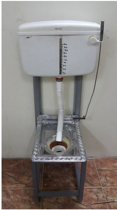
Fig. 8 The experimental setup for the proposed rotatable trapway system
